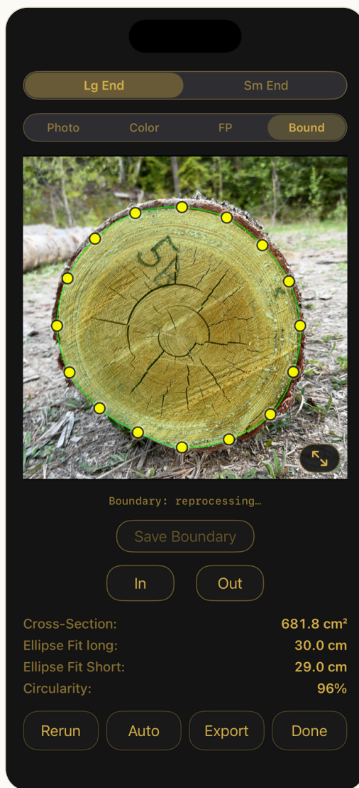
The Bound tab after manual boundary editing. Sixteen yellow handles ring the detected edge; the status reads Boundary: reprocessing... . All four action buttons ( Rerun / Auto / Export / Done ) are visible — Rerun has activated now that a manual edit exists on file.
